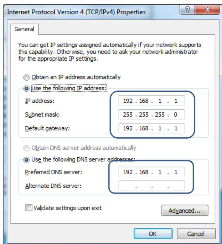
Connect the RJ45 Ethernet (LAN) cable between PC and MB2 controller after setup the TCP/IPv4. And go to "Preferences" → "Communication" and confirm the checked sign ✓ in the default box, then click "Done" button to close.
