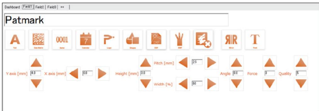
By clicking on a field, the properties panel opens and allows adjustment to the character height, marking force and quality, XY position and more settings such as serial settings.
