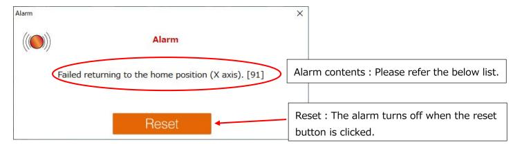
Also, the content of the alarm will be displayed at the bottom left of the screen of PM Win Software.
